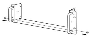
② Remove the handles from bottom bar. And turn the handles upside down, then replace the handles right side and left side.
