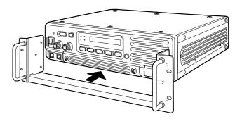
(3) Tighten the 1 supplied screws (M4  $\times$  8) and 2 removed screws to each side. (6 screws at total)
