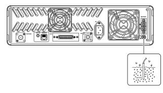
**WARNING: NEVER** connect the [GND] terminal to a gas or electric pipe, since the connection could cause an explosion or electric shock.
